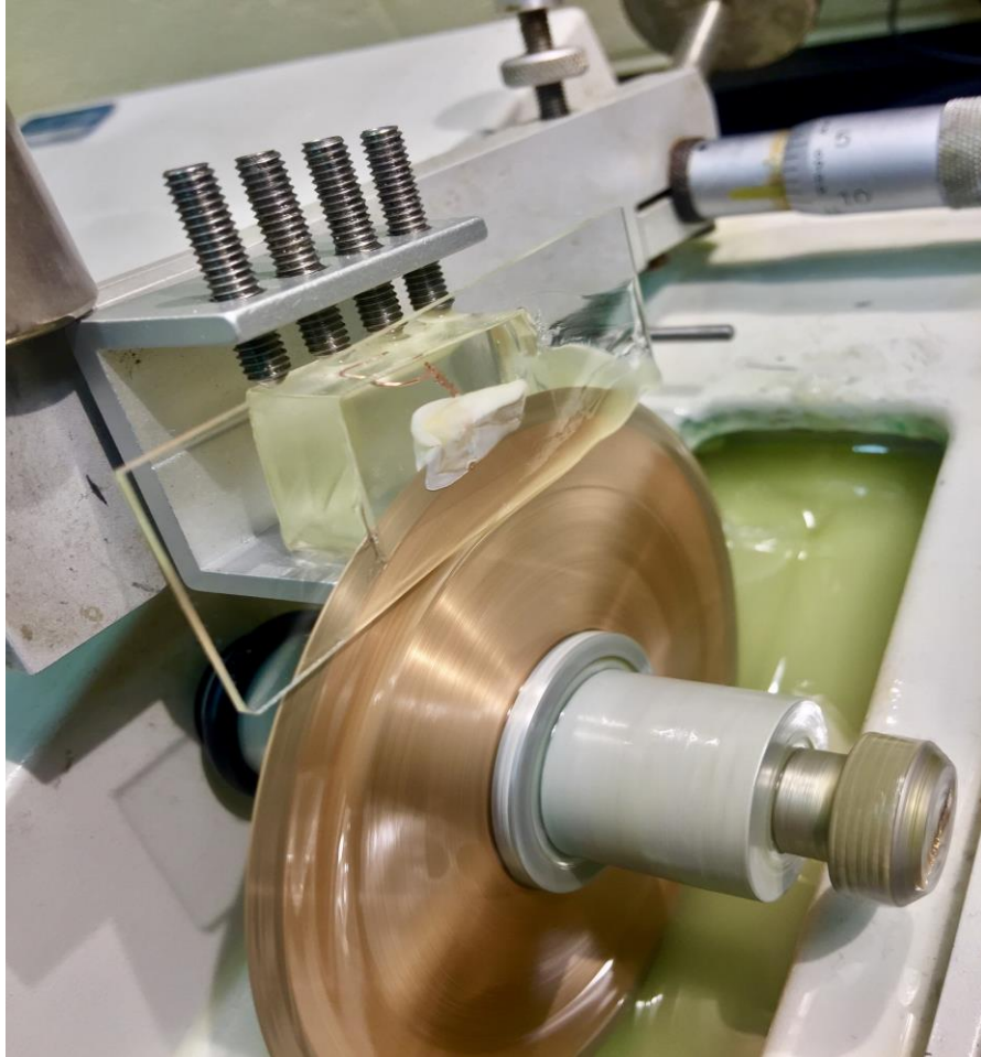
Figure 5.5 Photograph of longitudinal thin section being made.
