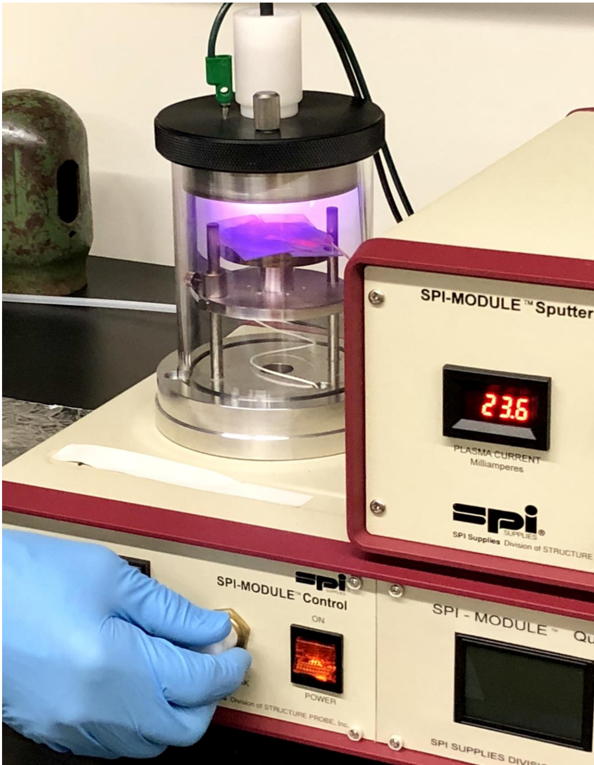
Figure 5.6 Photograph of thin section being coated in gold by sputter coater.
