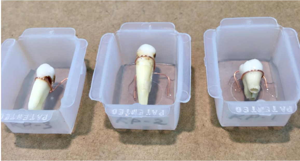
Figure 5.3 Photograph of teeth being prepared of embedding, wrapped in copper wire and placed in molding trays.
