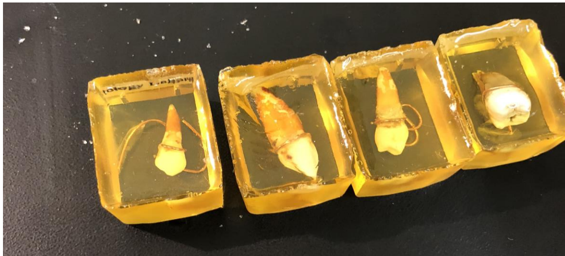
Figure 5.1 Photograph of embedded teeth used to take transverse thin sections, by Kortney Dewayne Powell.
