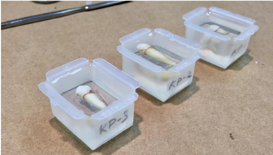
Figure 5.4 Photograph of teeth in molding trays, filled epoxy.
